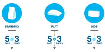
of bags maintained package integrity. Heavy duty sacks produced with SPsK919 will withstand the challenges and abuse of the modern supply chain.
