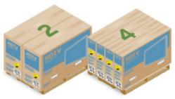
▲ Using conventional cushioning foam (left), a large flat-screen television with its stand can be packed with only two units to a standard pallet. Switching to ARCEL resin (right) and removing the stand allows for cartons approximately half the size, easily doubling
