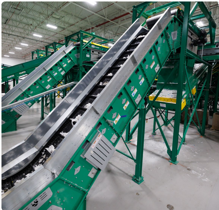
Photo of sorting equipment used in Connersville. Sorting is one of the first steps in the mechanical recycling process.
