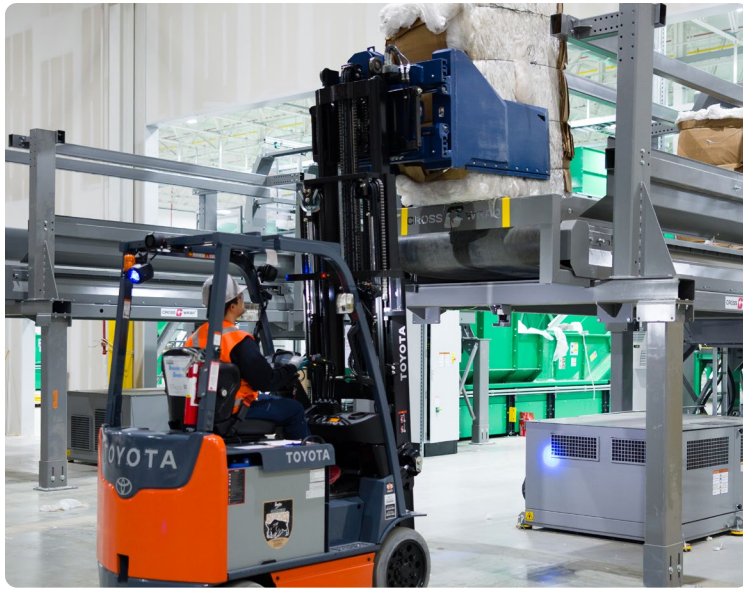
Before the mechanical recycling process begins, bales of post-consumer plastic film are loaded onto the processing line. These bales are placed onto a conveyor belt using forklifts, where bale breakers open them up so the plastics can move freely into the sorting system.
