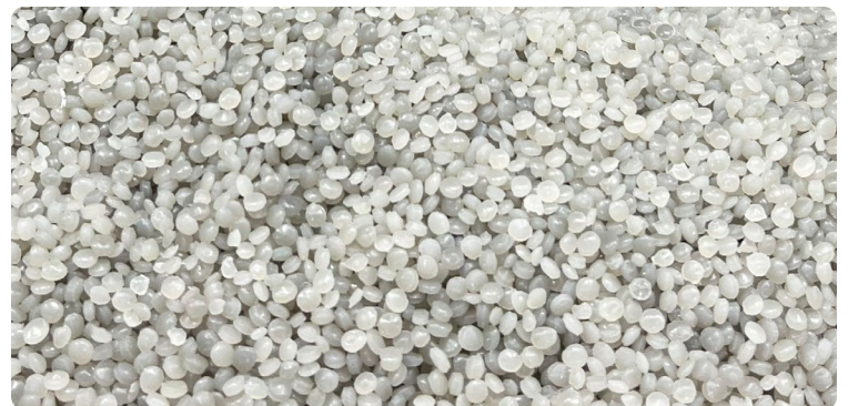
Photo of the SYNDIGO recycled polyethylene resins made in Connersville. These pellets can be used to create new recycled packaging for e-commerce, pet food, mulch and everyday packaging you find in the grocery store.
