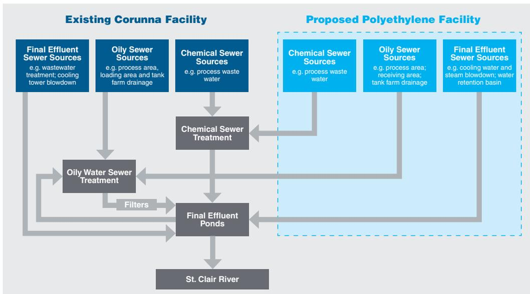
*This chart provides an overview of the waste water collection and treatment system for our existing Corunna facility, and the planned enhancements / tie-ins to the system if our proposed polyethylene facility goes ahead.*
