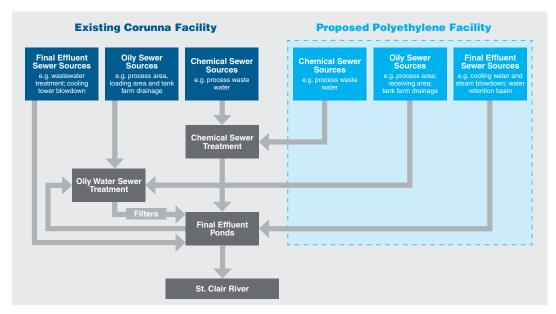
This chart provides an overview of the waste water collection and treatment system for our existing Corunna facility, and the planned enhancements / tie-ins to the system if our proposed polyethylene facility goes ahead.
